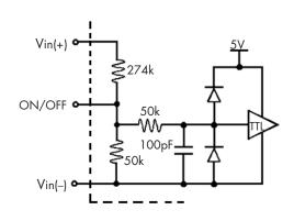
Figure B: Internal ON/OFF pin circuitry
