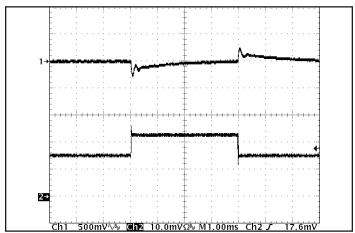
Figure 12: Output voltage response to step-change in load current (50%-75%-50% of lout(max):  $dI/dt = 1~A/\mu s$ ). Load cap:  $90~\mu F$ ,  $15~\mu F$ ,  $100~m\Omega$  ESR tantalum cap and  $1~\mu F$  cermaic cap. Ch 1: Vout (500 mV/div). Ch 2: lout (1 A/div).
