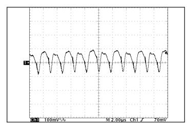
Figure 16: Output voltage ripple at nominal input voltage and rated load current (100 mV/div). Load capacitance: 1  $\mu F$  ceramic capacitor and one 15  $\mu F$ tantulum capacitor. Bandwidth: 20 MHz. See Figure 13.
