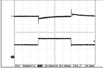
Figure 11: Output voltage response to step-change in load current (50%-75%-50% of lout(max); dI/dt = 0.1 A/ $\mu$ s). Load cap: 15  $\mu$ F, 100 m $\Omega$  ESR tantalum cap and 1  $\mu$ F cermaic cap. Ch 1: Vout (500 mV/div). Ch 2: Iout (1 A/div).
