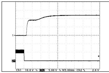
Figure 10: Turn-on transient at zero load (5 ms/div). Ch 1: Vout (10 mV/div). Ch 2: ON/OFF input (5 V/div)
