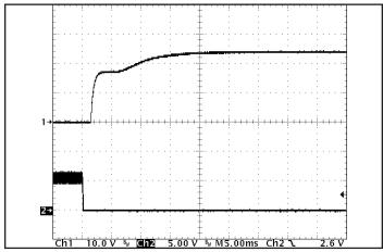
Figure 9: Turn-on transient at full load (resistive load) (5 ms/div). Input voltage pre-applied. Ch 1: Vout (10 mV/div). Ch 2: ON/OFF input(5 V/div)
