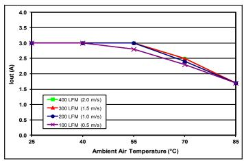
Figure 7: Maximum output power derating curves vs. ambient air temperature for airflow rates of 100 LFM through 400 LFM with air flowing lenghtwise from input to output (nominal input voltage).
